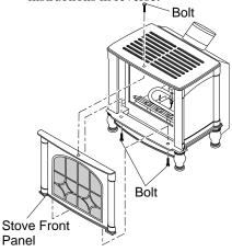
Figure 49 - Removing Front Panel from Stove
